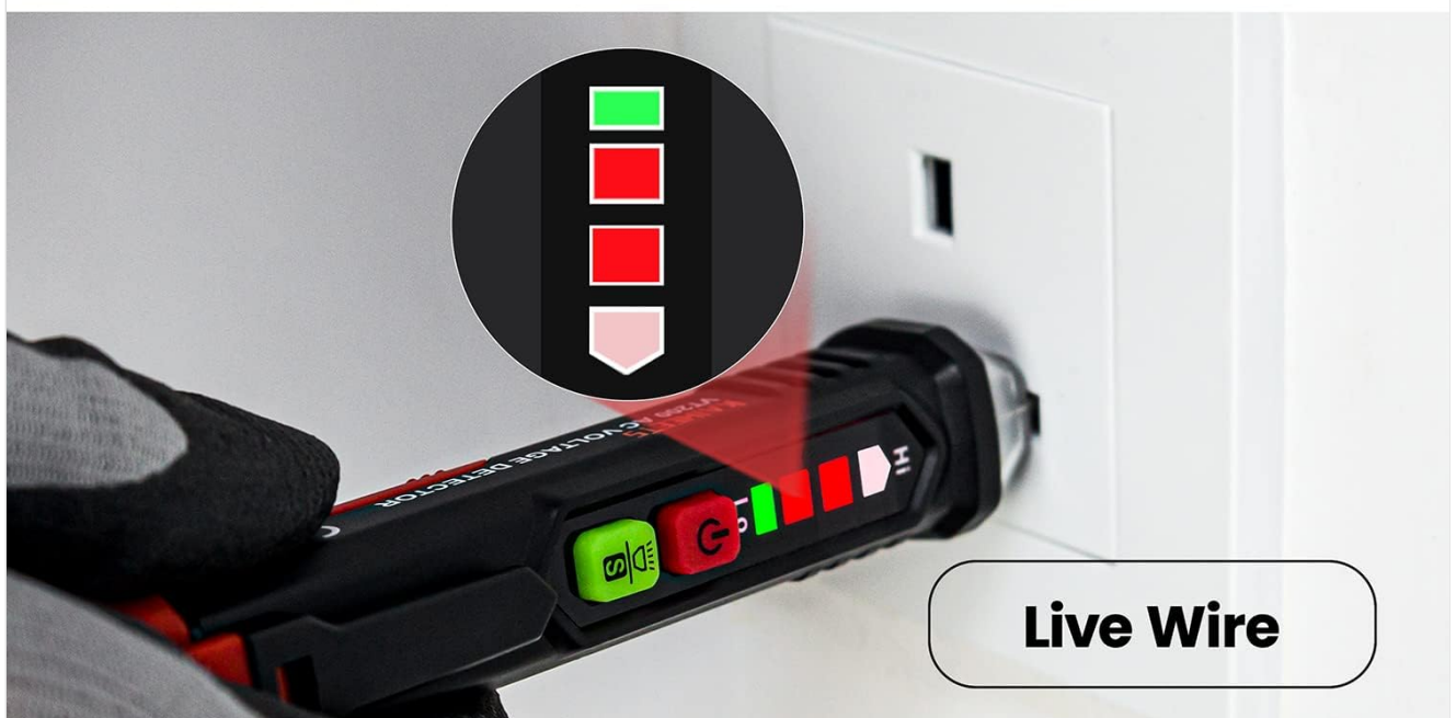
Figure 4: Live and Neutral Wire Detection
