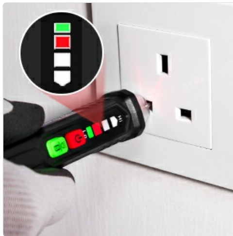
Figure 13: Neutral Wire Indication
