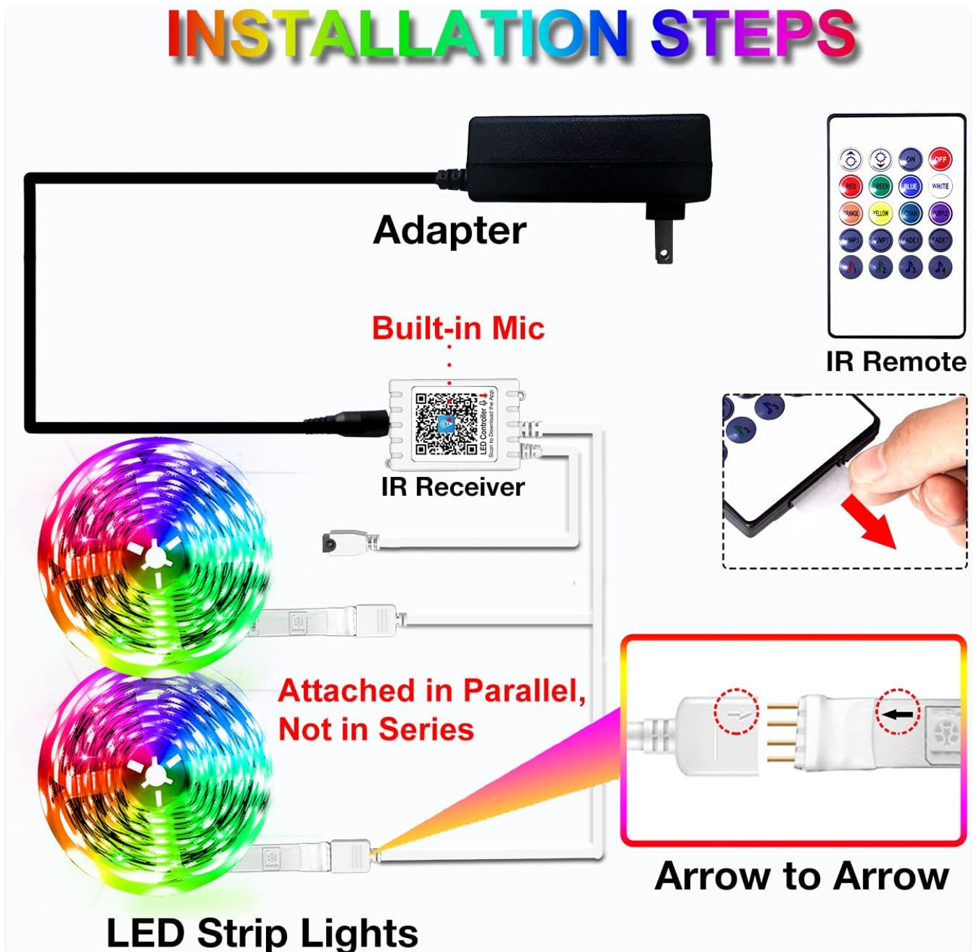
Image 3.1: Installation Steps. Note that the two 50ft rolls are attached in parallel, not in series, to the IR receiver.
