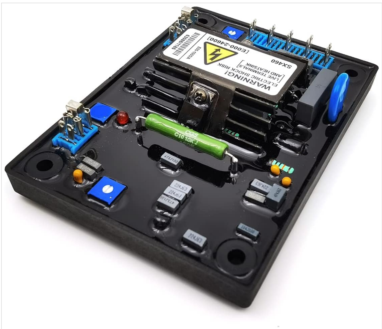
Image: Another top view of the DEVMO SX460 AVR, showing the layout of the circuit board.
