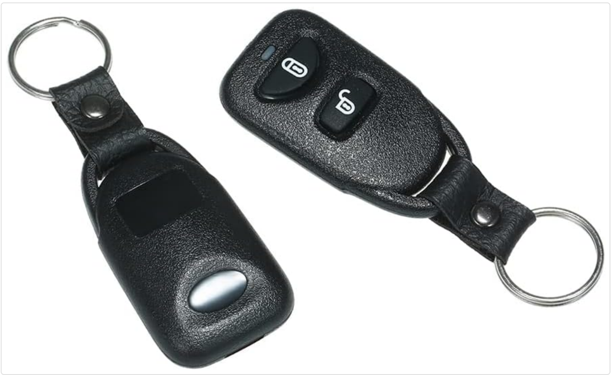
Figure 2.2: Two remote control key fobs for the central locking system. Each fob features lock and unlock buttons.
