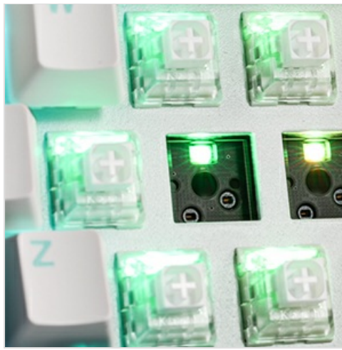
Image: A detailed view of the hot-swappable switch sockets on the keyboard, showing how switches can be easily removed and replaced without soldering.
