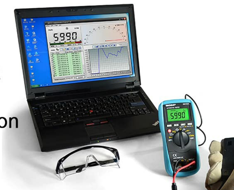
Figure 5.13: Diagram showing the allsun EM133A multimeter connected to a laptop via a USB cable for data transfer.
