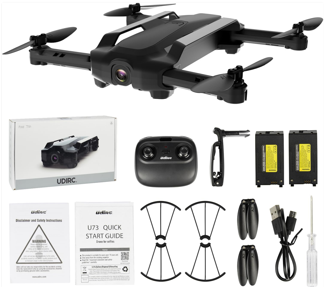
Figure 2.1: All components included in the Cheerwing U73 Mini Drone package.
