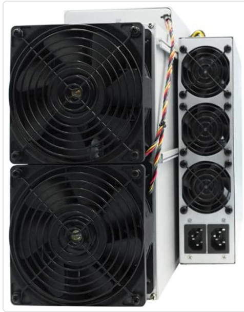
Figure 3.2: Close-up front view of the Antminer S19jpro+, highlighting the dual large cooling fans.
