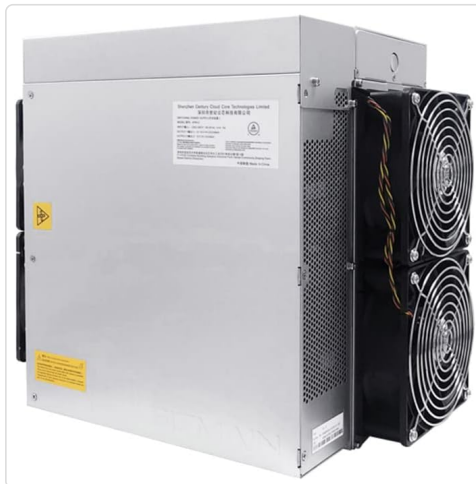
Figure 3.3: Rear and side view of the Antminer S19jpro+, showing the exhaust fans and network port.
