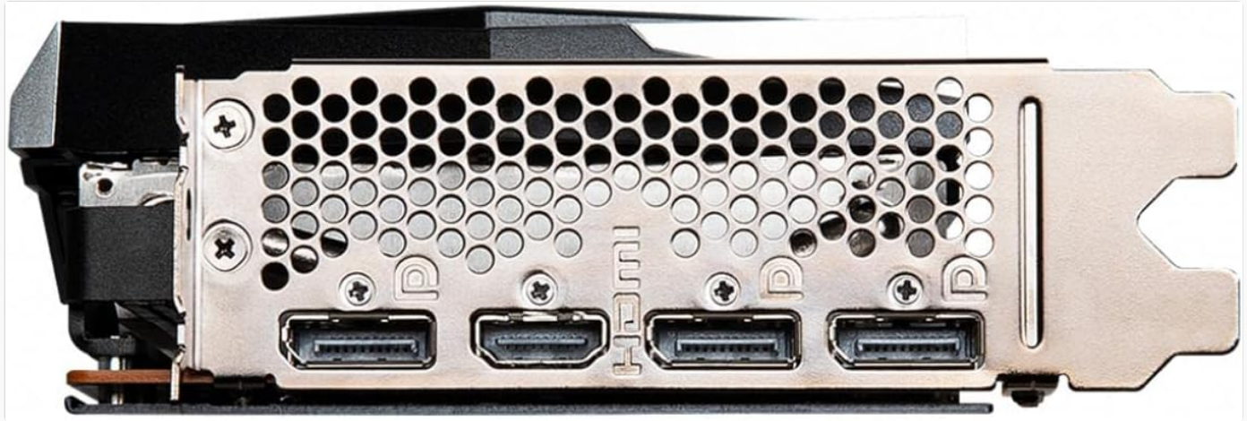
Image: Rear view of the graphics card showing three DisplayPort (v1.4) and one HDMI output.
