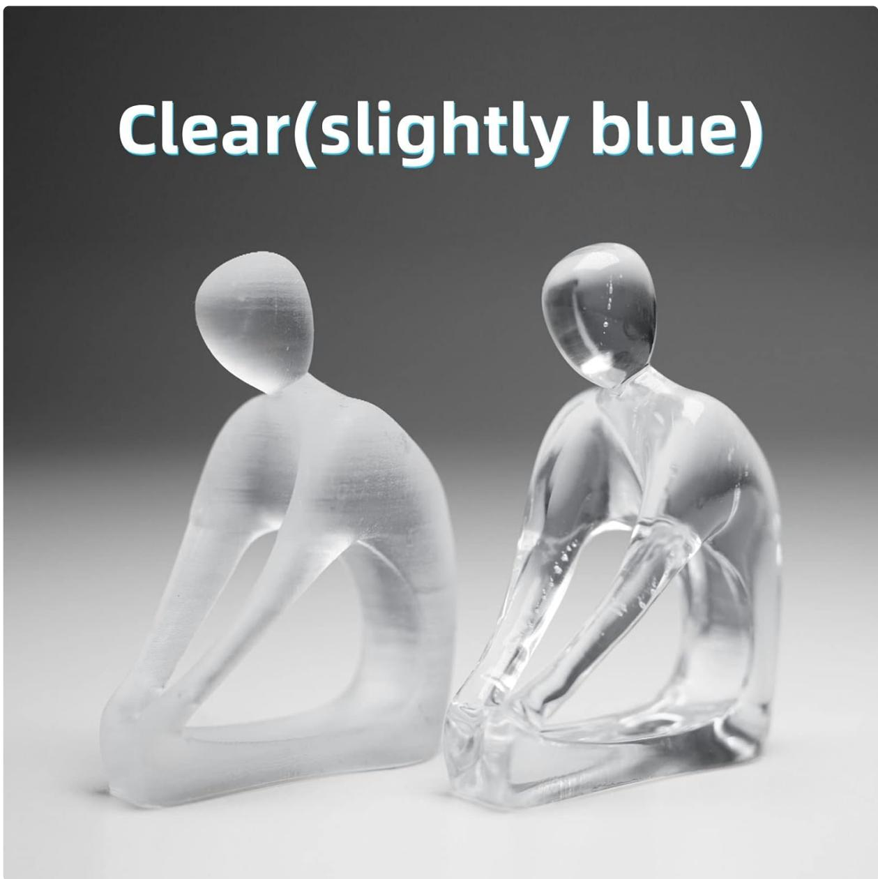
Demonstration of G217 resin's clarity, showing a frosted print before clarity enhancement and a clear print after.
