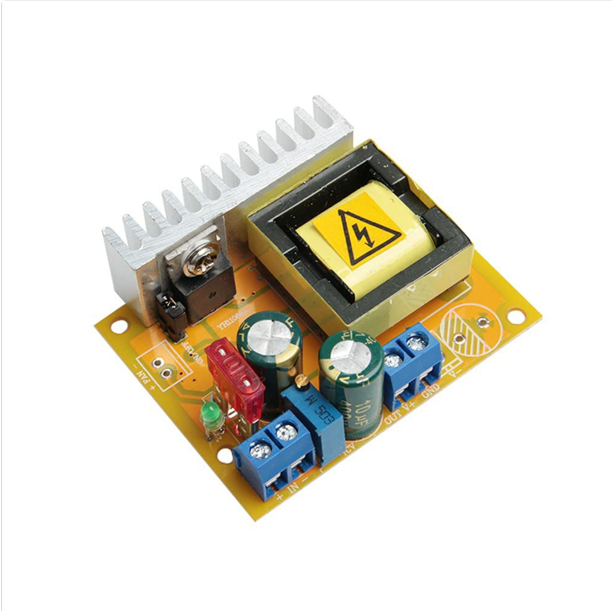
Figure 1: Top view of the Acxico DC-DC Boost Converter module. This image highlights the input terminals (8-32V), output terminals (+45-390V), the output voltage regulation potentiometer, and fan connectors. The large transformer and heatsink are also visible.
