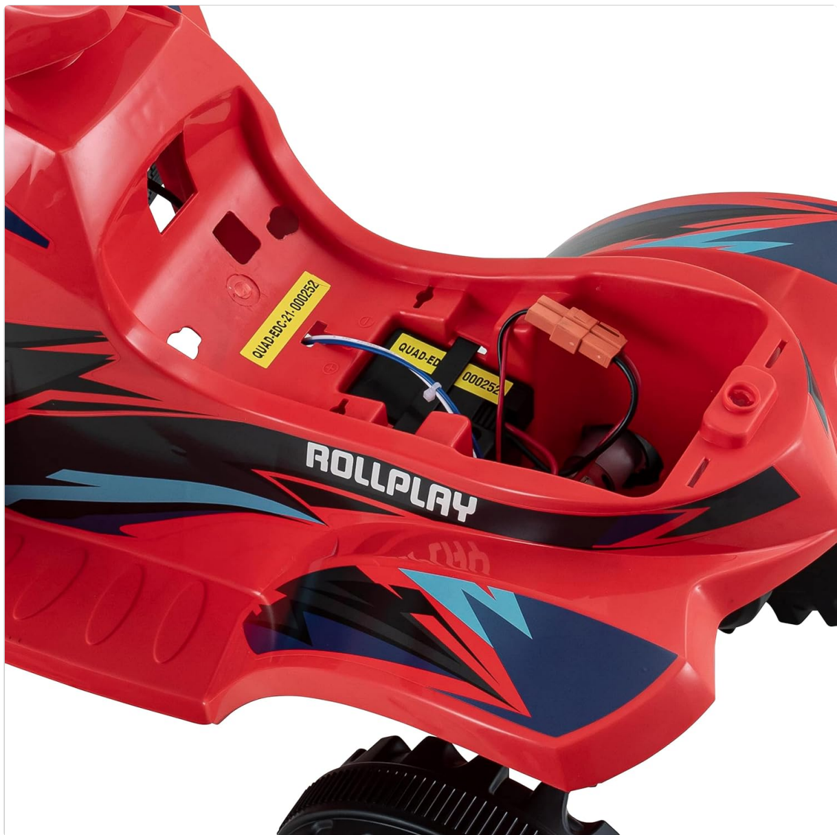
Image 4.1: View of the battery compartment, showing the location for battery connection.
