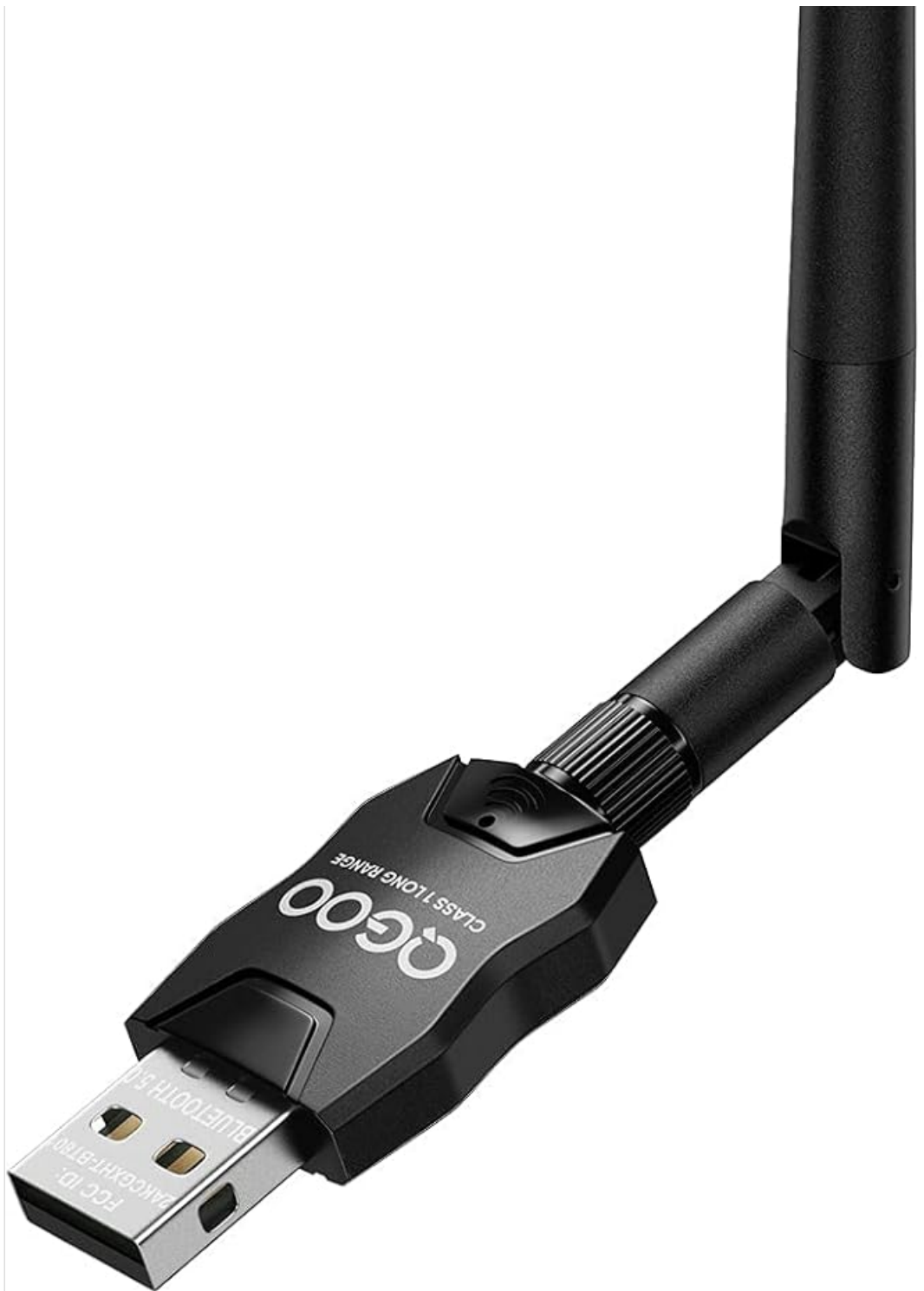
Figure 1: QGOO Long Range Class 1 Bluetooth Adapter with antenna.
