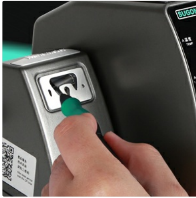
Figure 5.1: Proper insertion of a soldering iron tip into the handle.
