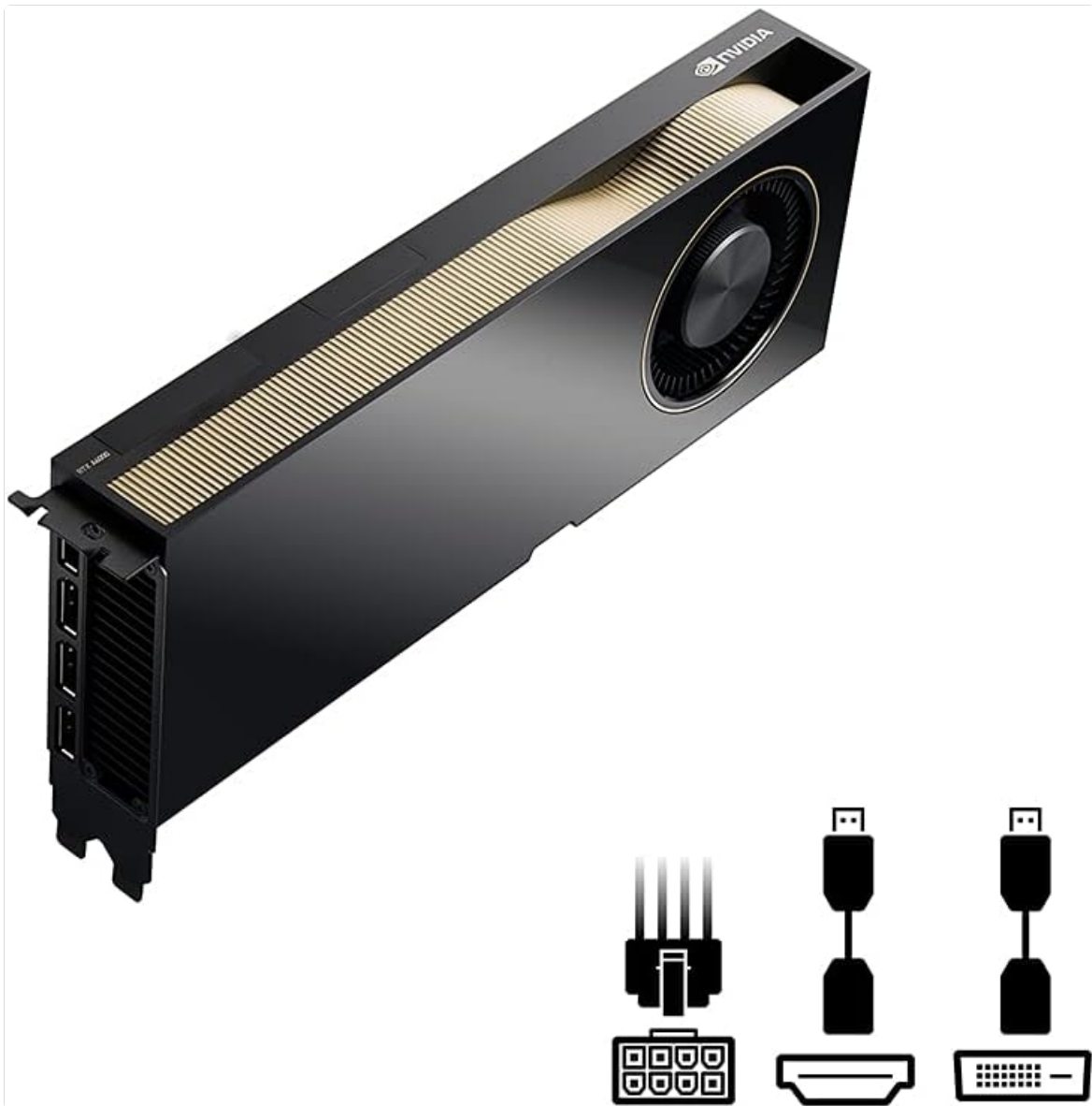
Figure 3.1: Graphics card with illustrations of power and display connectors. This image highlights the necessary power input and common display output types (HDMI, DisplayPort) for the graphics card.
