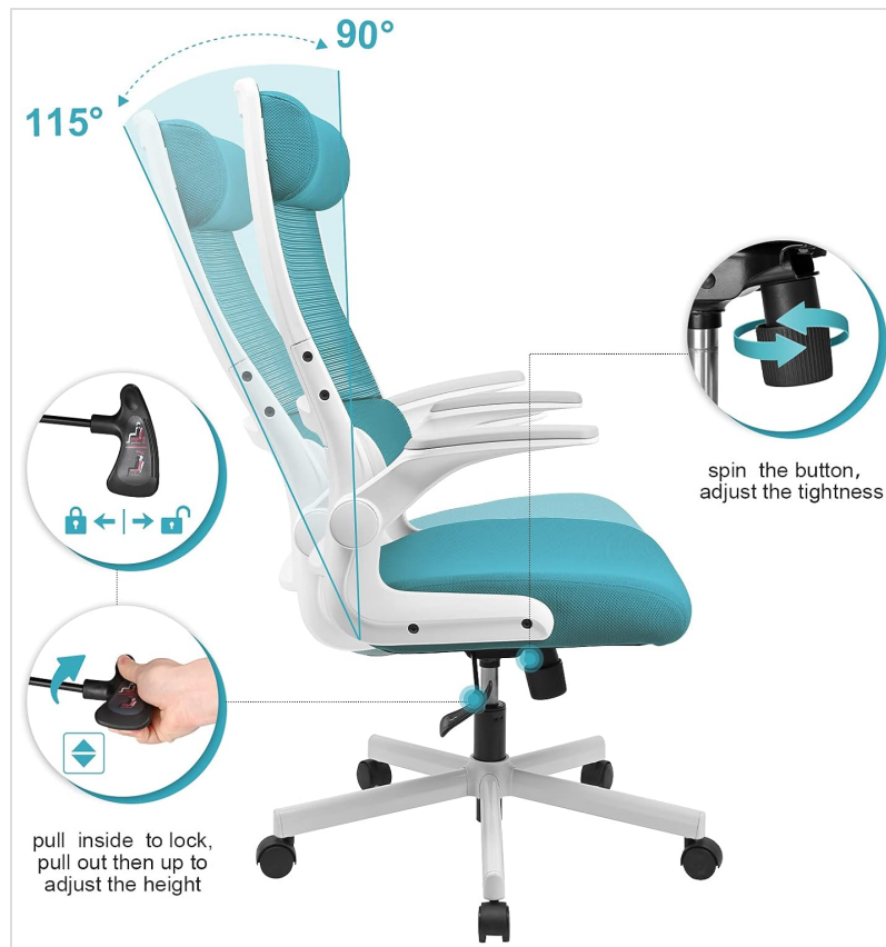
Image: Chair Adjustments. This diagram illustrates how to adjust the chair's height using the lever and the tilt tension using the knob.
