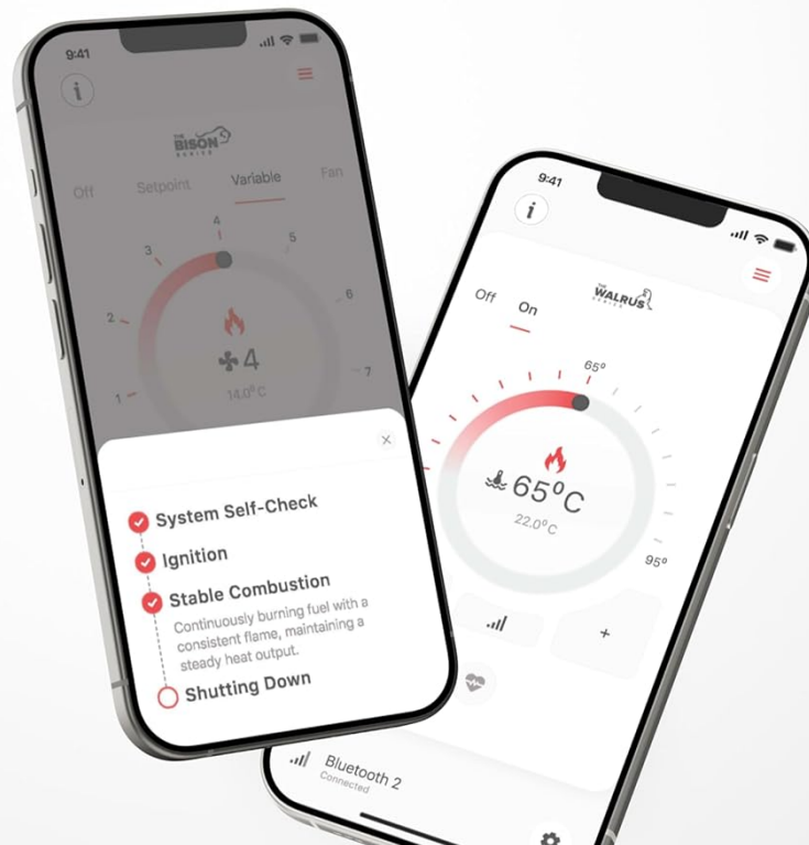
Figure 5.1: Screenshots demonstrating the General Components mobile application interface for controlling the heater, including system self-check and temperature settings.
