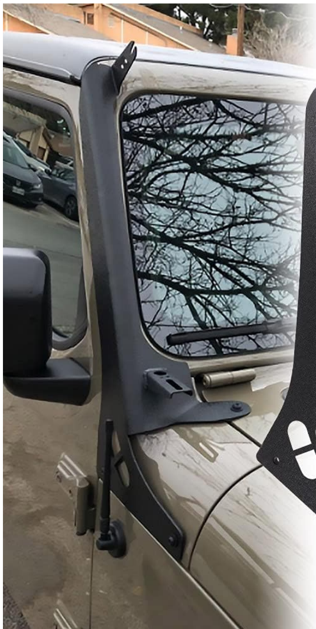
Image 1.1: Samman 52-inch LED Light Bar Upper Windshield Mounting Brackets. This image displays the two black, textured metal brackets designed for mounting a light bar on a vehicle's windshield frame.
