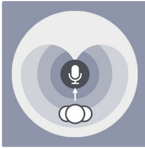
Image: Visual representation of the Cardioid pickup pattern, focusing on sound from the front.
