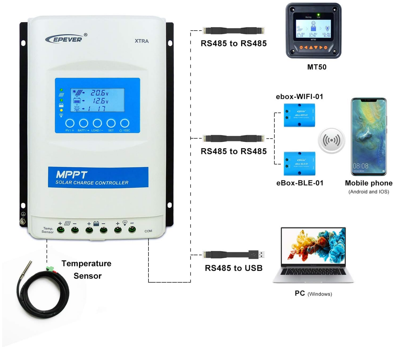
Connection diagram for the EPEVER MPPT Solar Charge Controller.
