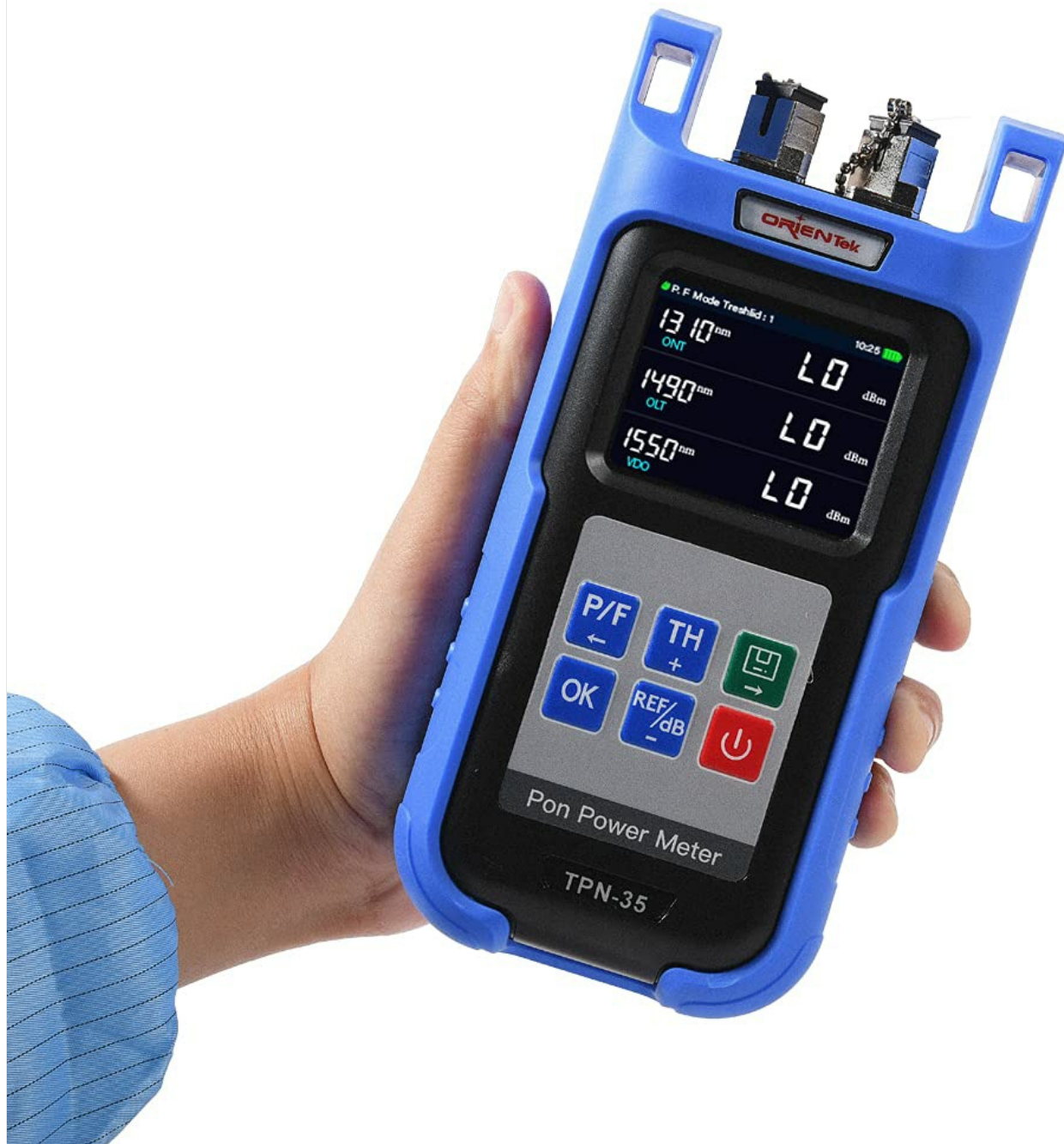
Figure 6.2: The TPN-35 display showing simultaneous power measurements for multiple wavelengths.
