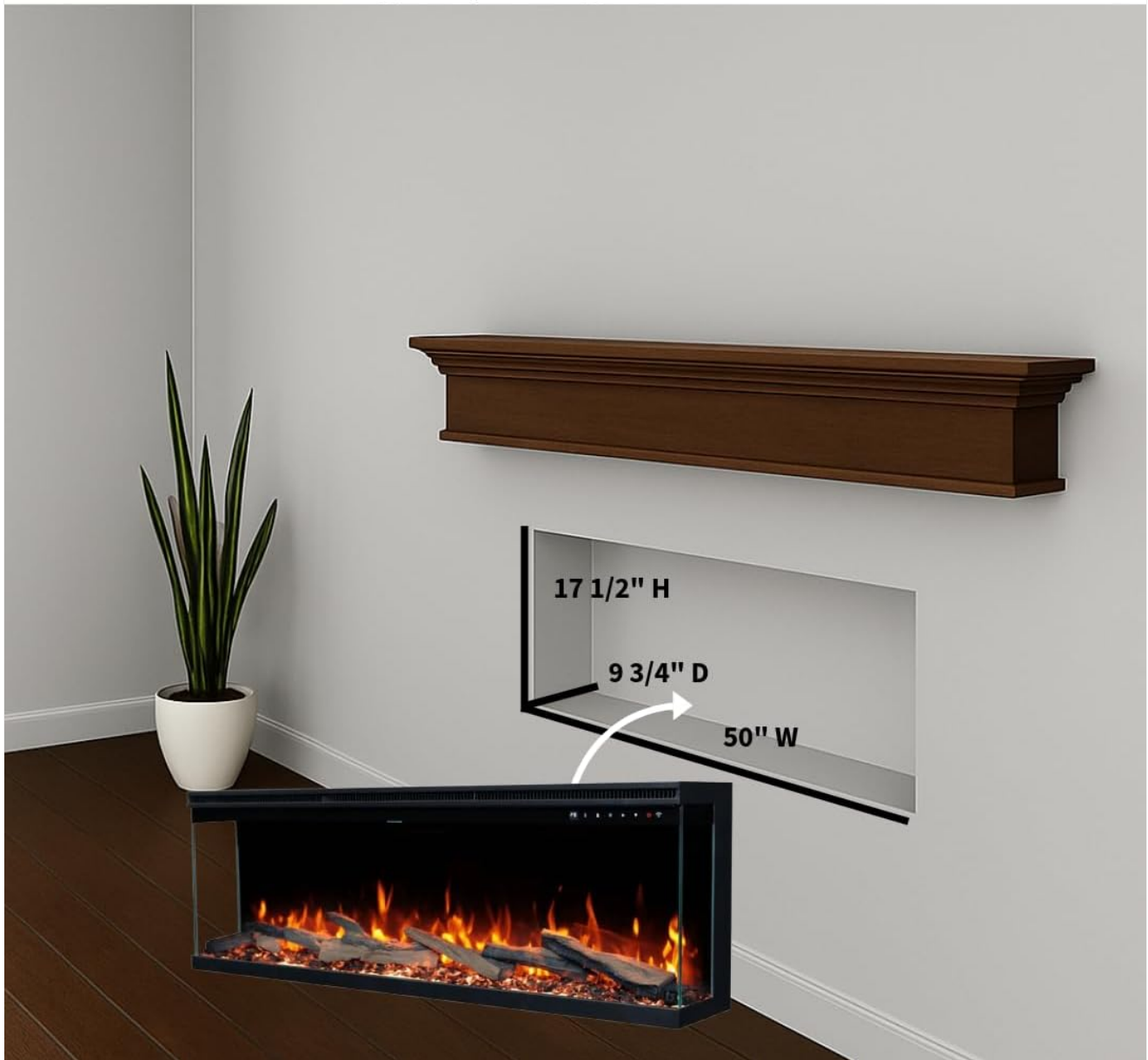
Image 4: Diagram illustrating the required rough opening dimensions for built-in installation.
