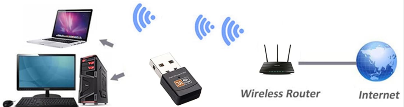
Figure 5.1: Diagram illustrating both AP Mode (transmitting Wi-Fi from a wired connection) and Station Mode (receiving Wi-Fi from a wireless router).
