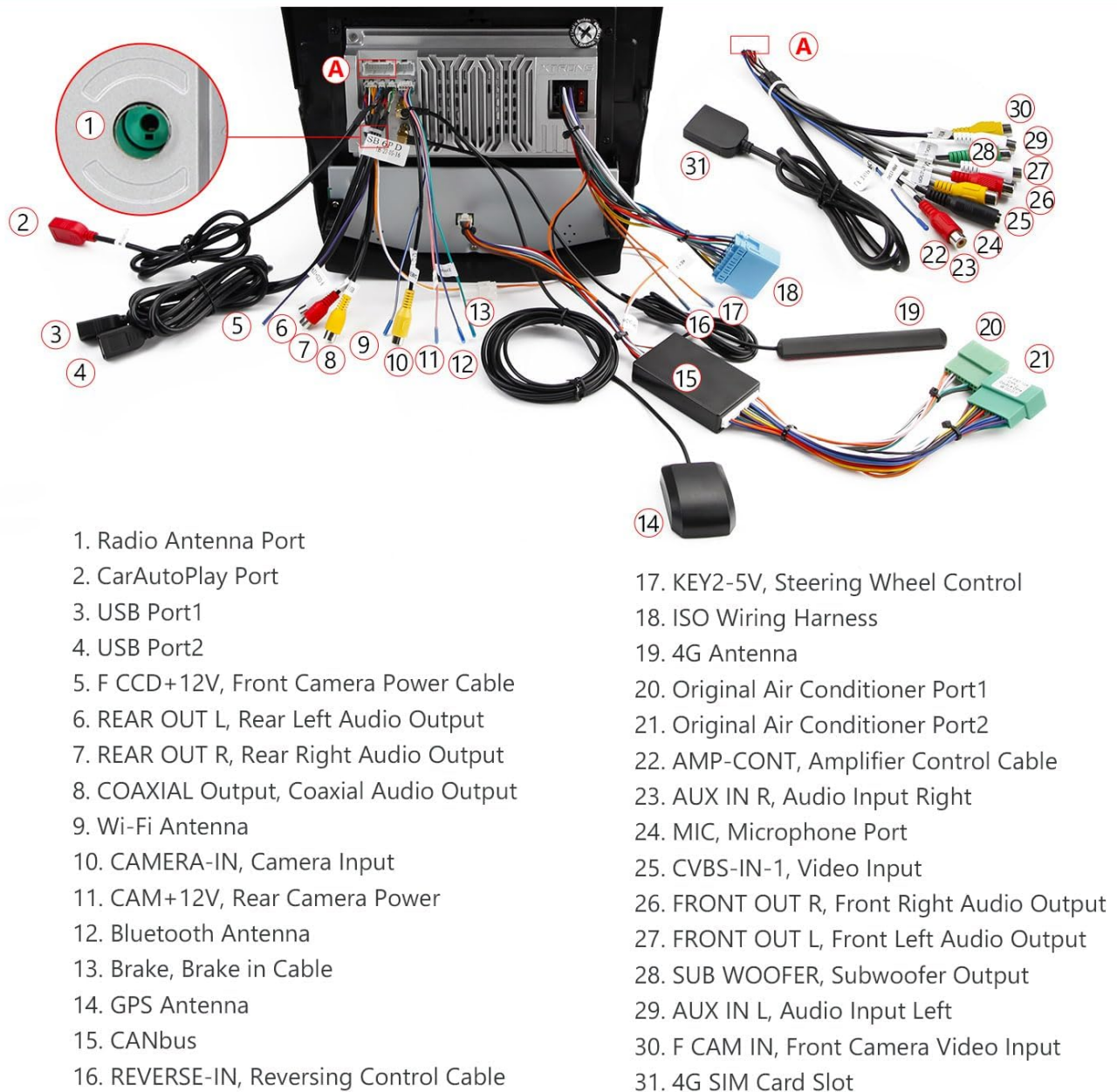
Figure 4.1: Wiring Diagram for XTRONS Car Stereo
