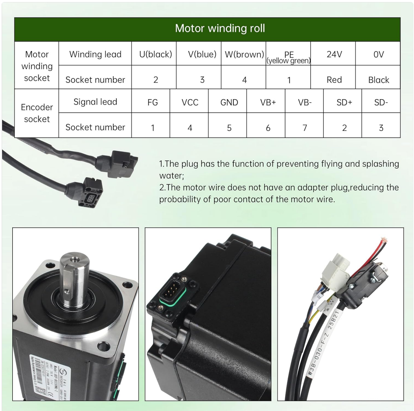
Figure 5.1.3: Motor Winding and Encoder Socket Wiring.
