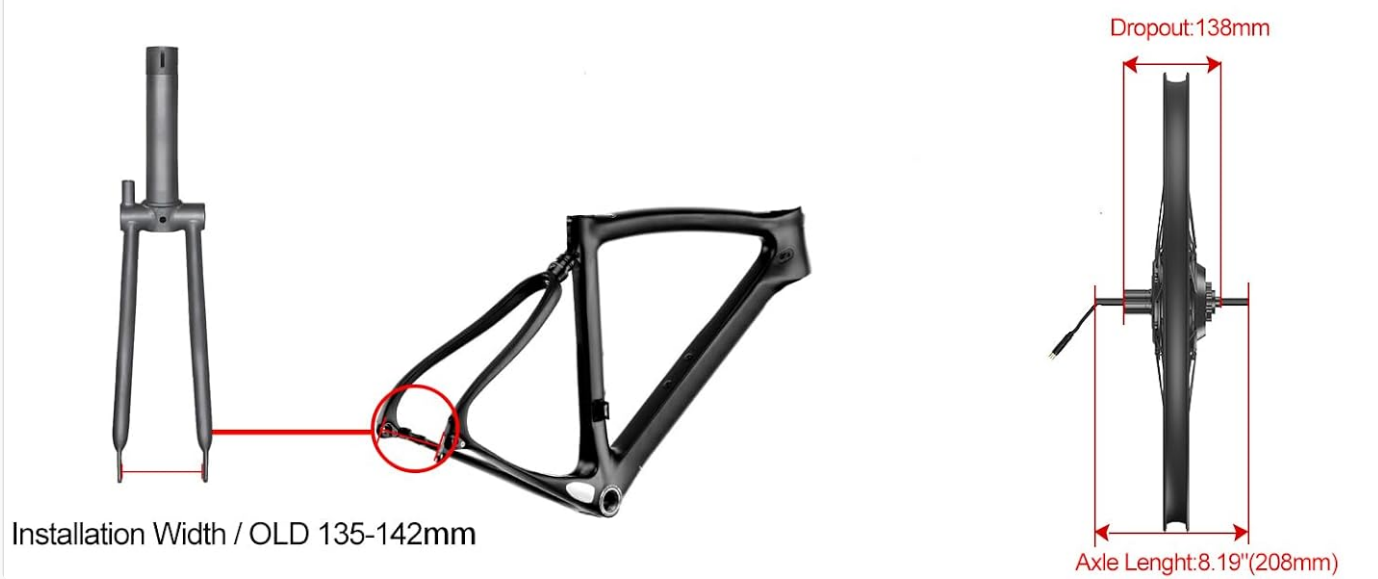
Image 2.2: Diagram illustrating various wheel size options and frame compatibility requirements, including the rear dropout measurement (OLD 135-142mm).
