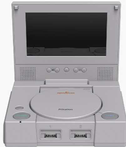
Figure 2.2: Close-up of the integrated 4.3-inch LCD screen with control buttons for volume, screen brightness, and aspect ratio switching, flanked by stereo speakers.
