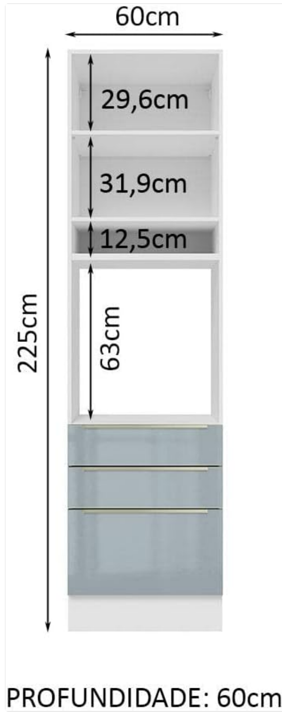
Image 4.1: Internal dimensions of the Madesa Lux 60 cm Hot Tower.
