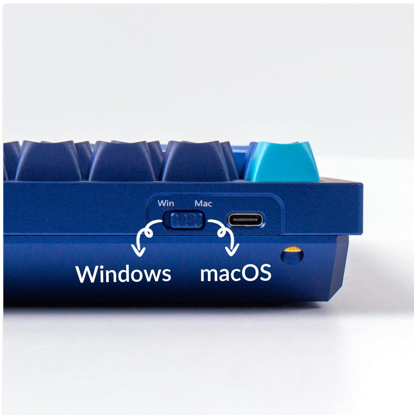
Image: Close-up of the Keychron Q1 V2 keyboard's side, showing the physical switch to select between Windows and macOS modes.
