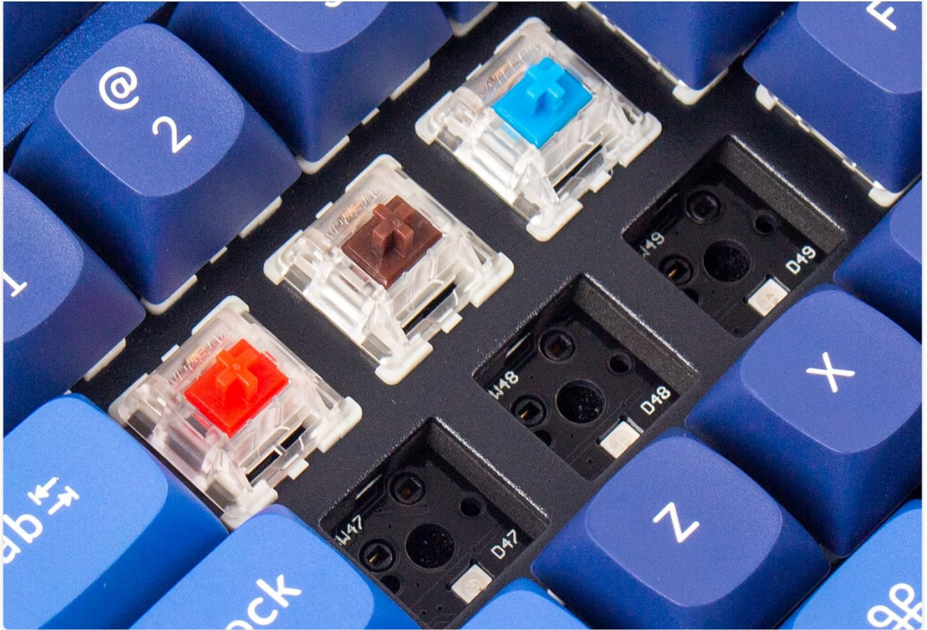
Image: Close-up view of the keyboard's PCB with several switches removed, illustrating the hot-swappable sockets for easy switch replacement.
