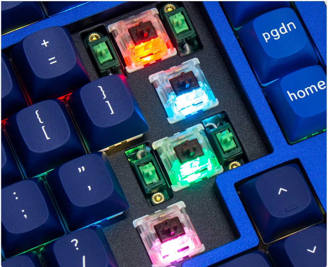
Image: Close-up of the keyboard's switches with RGB backlighting active, demonstrating the south-facing LED orientation.
