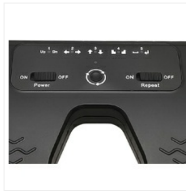
Image 3.2: Control panel with power, repeat, and mode selection buttons.
