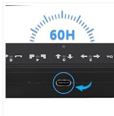
Image 2.2: Detail of the Type-C charging port.
