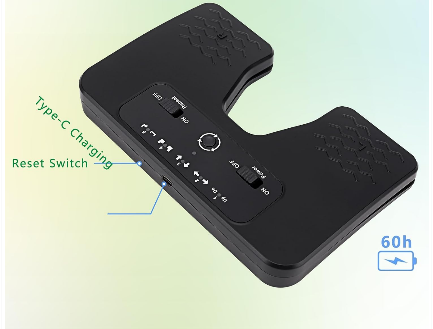
Image 2.1: Location of the Type-C charging port and reset switch.
