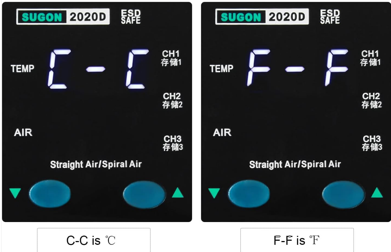
Figure 6.2: Temperature Unit Switching. This image illustrates the display showing "C-C" for Celsius and "F-F" for Fahrenheit, indicating the selected temperature unit.
