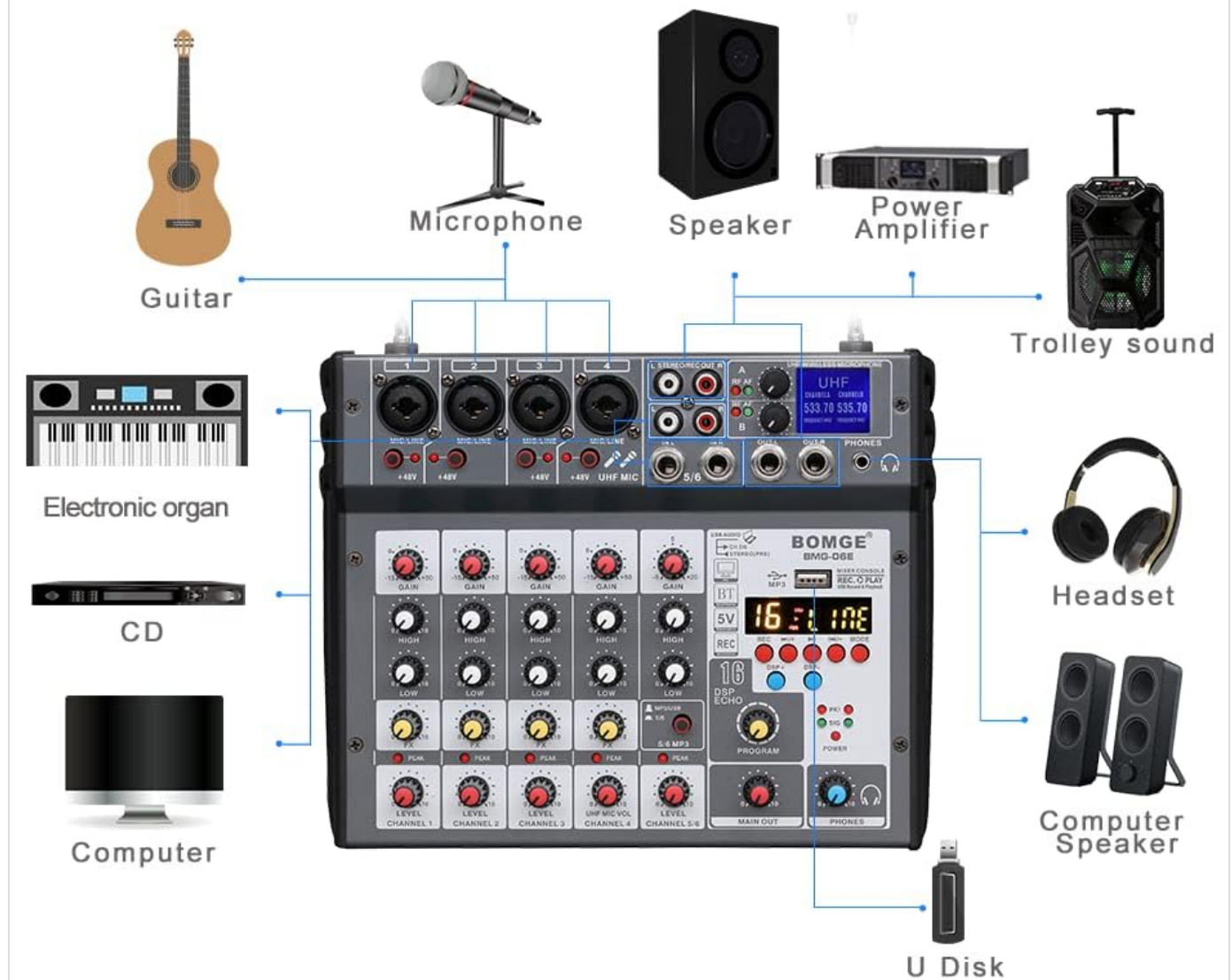
Figure 2: Connection diagram for various devices including guitars, microphones, speakers, and computers.
