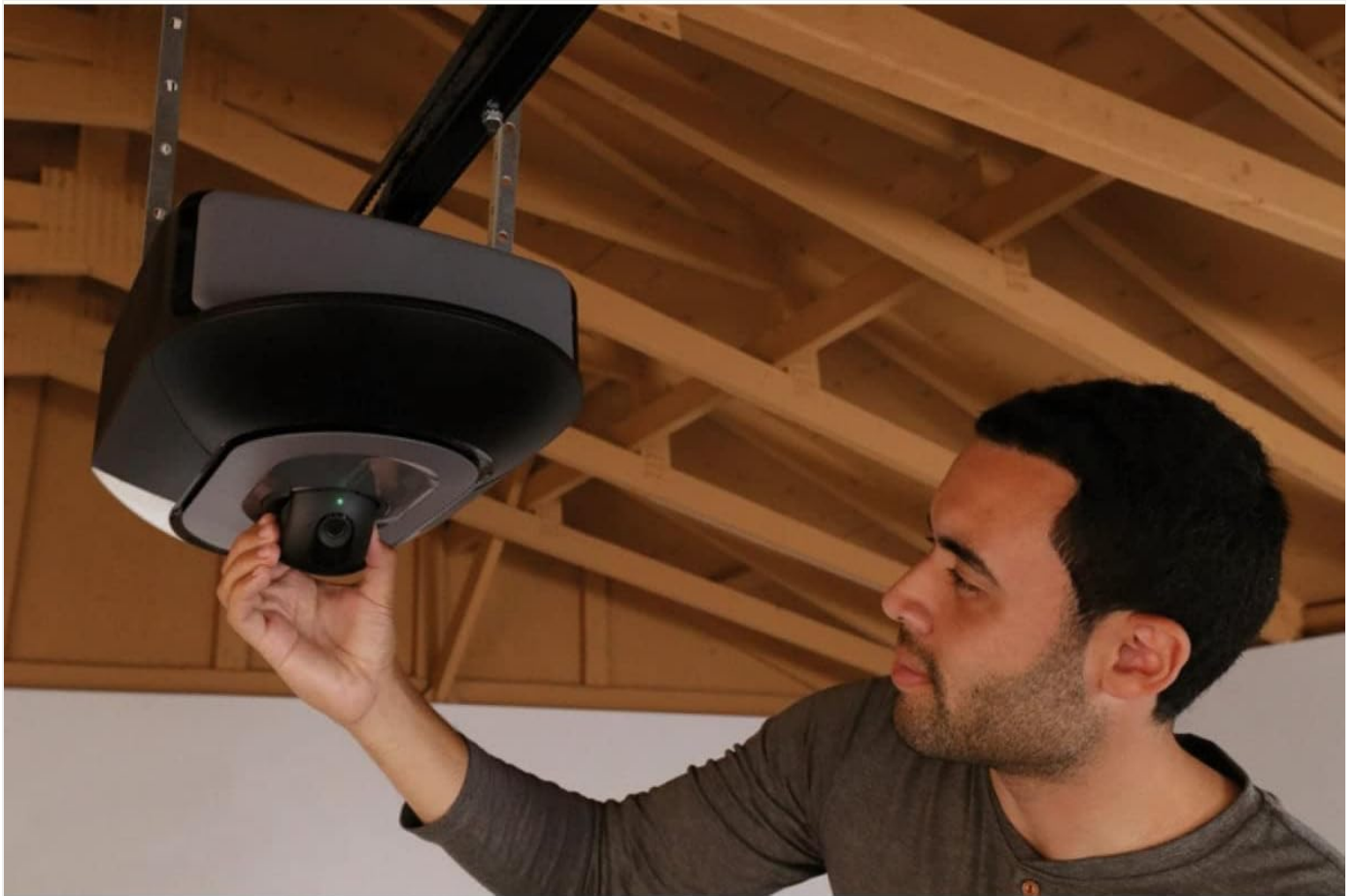
Figure 3: Adjusting the integrated camera after installation.
