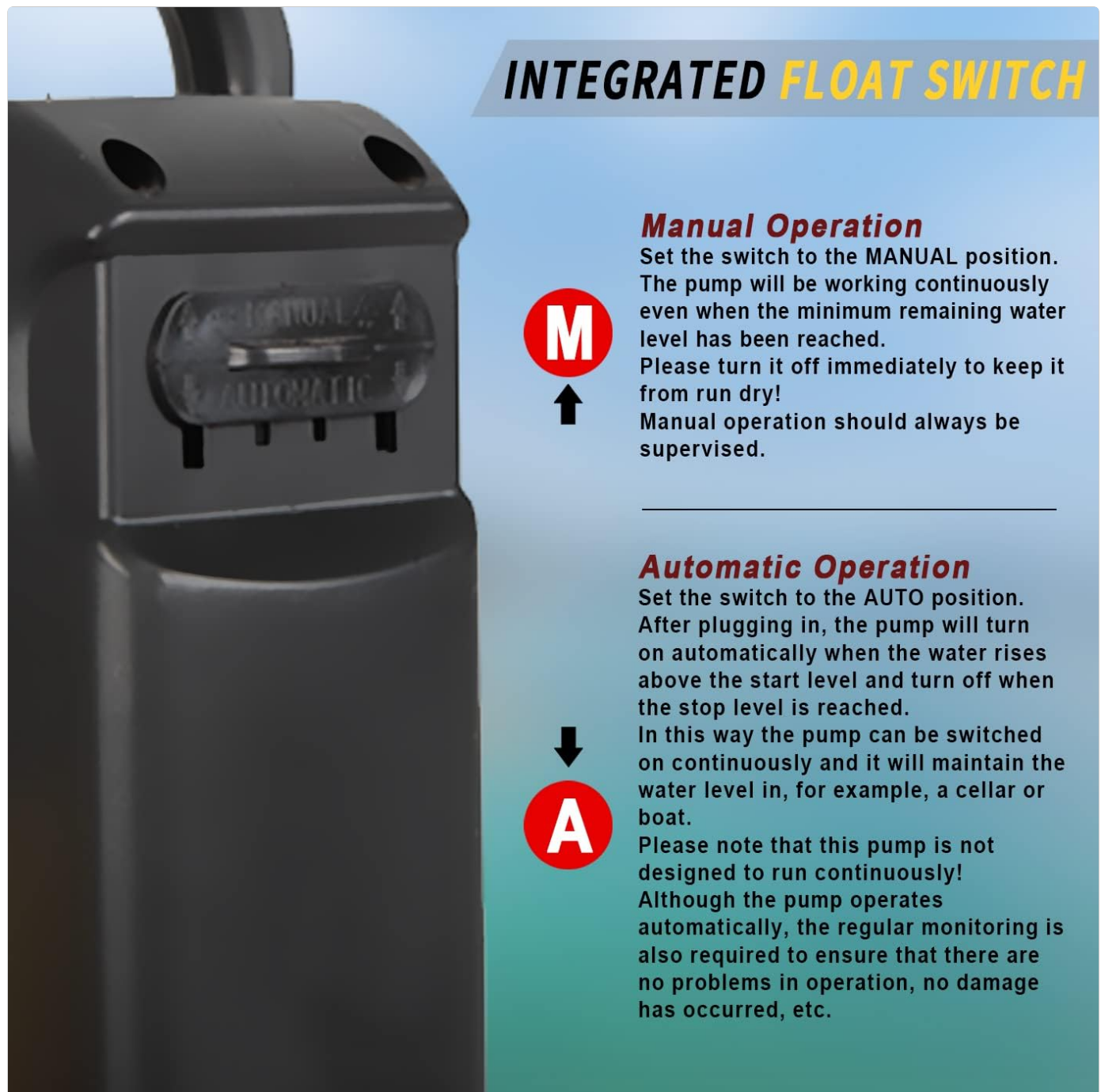
Figure 6: Integrated float switch operation modes.
