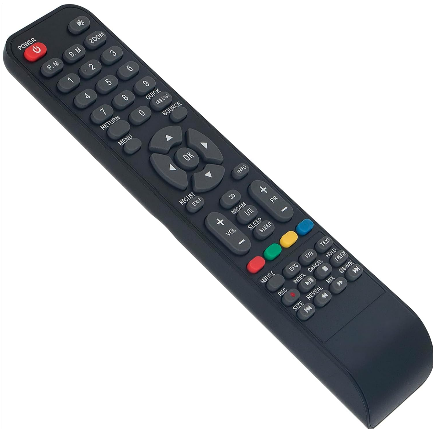
Figure 1: Front view of the ALLIMITY replacement remote control. This image displays the layout of all buttons, including power, number keys, navigation, volume, channel, and special function buttons.
