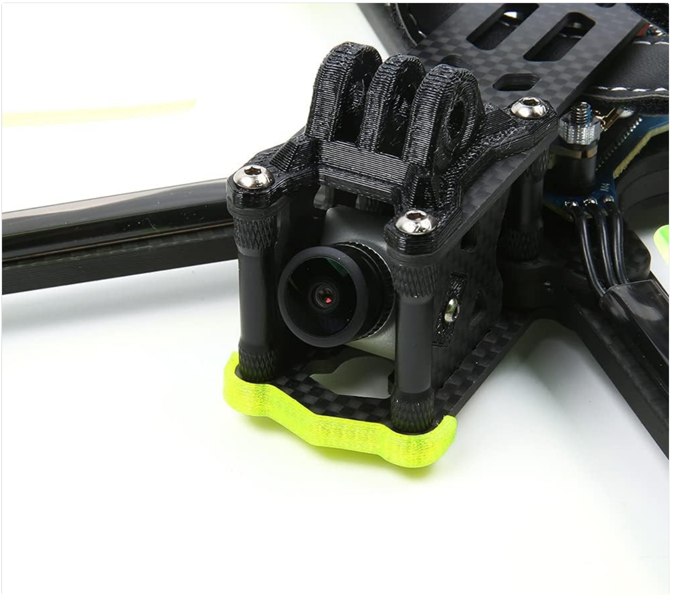
Figure 2: Close-up view of the Caddx Polar camera module integrated into the drone's front section. This camera provides the digital high-definition video feed.
