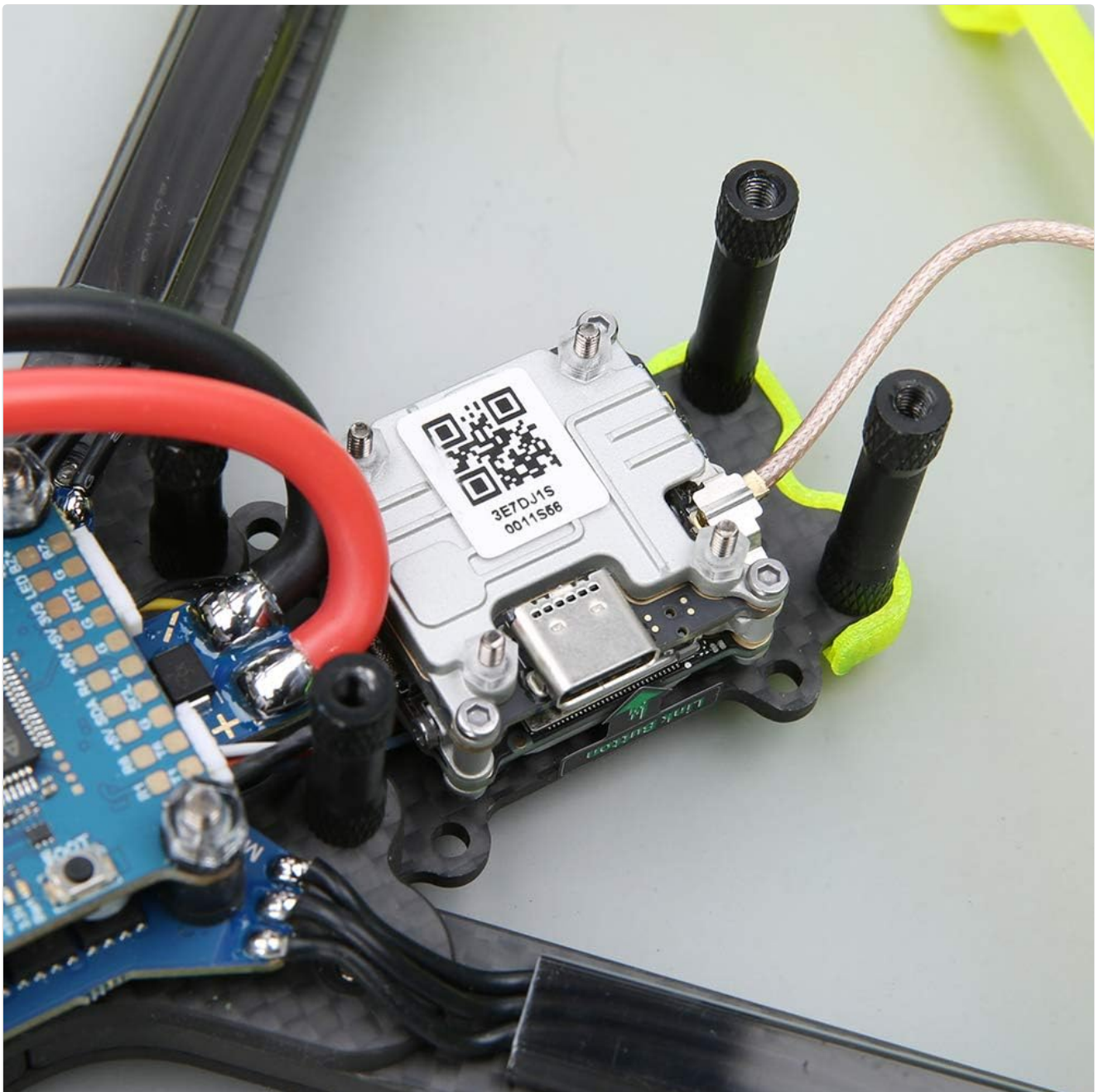
Figure 3: The Caddx Polar Vista Digital HD System unit mounted on the drone's frame. This unit processes and transmits the digital video signal to compatible FPV goggles.
