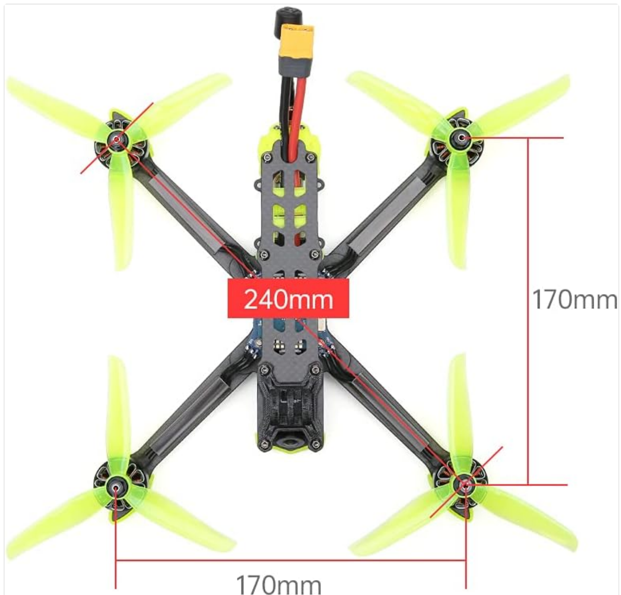
Figure 4: Dimensional overview of the iFlight Nazgul5 V2 HD Drone, indicating a frame width of 240mm and arm lengths of 170mm.
