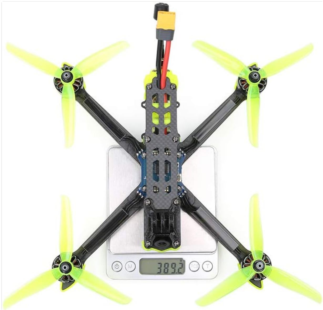
Figure 5: The iFlight Nazgul5 V2 HD Drone on a scale, showing a weight of 389.2 grams without battery.
