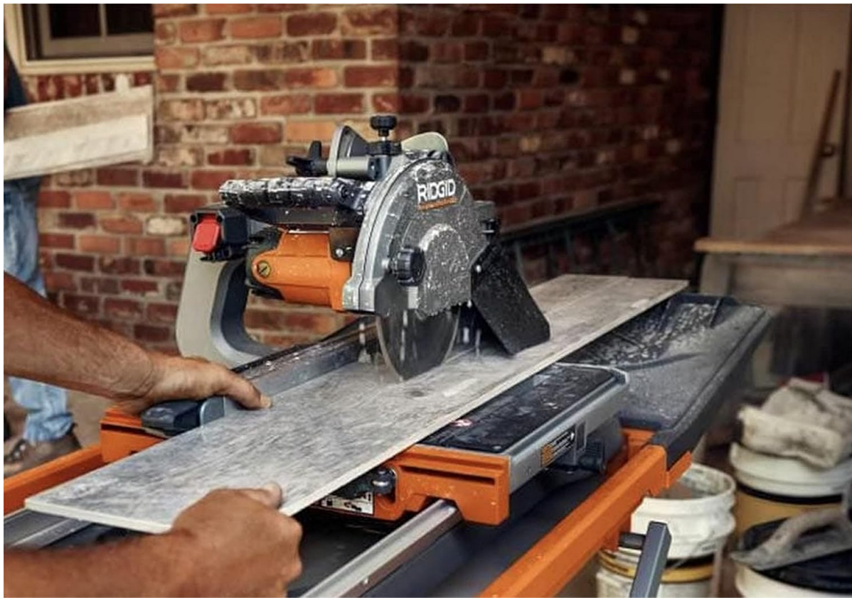
Figure 4.1: Proper technique for feeding a tile through the saw blade for a straight cut.
