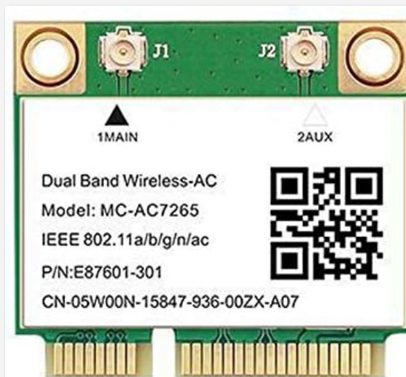
Image 1.1: Front view of the Teday MC-AC7265 Half Mini PCI-E WiFi Card, showing the main components and labels.
