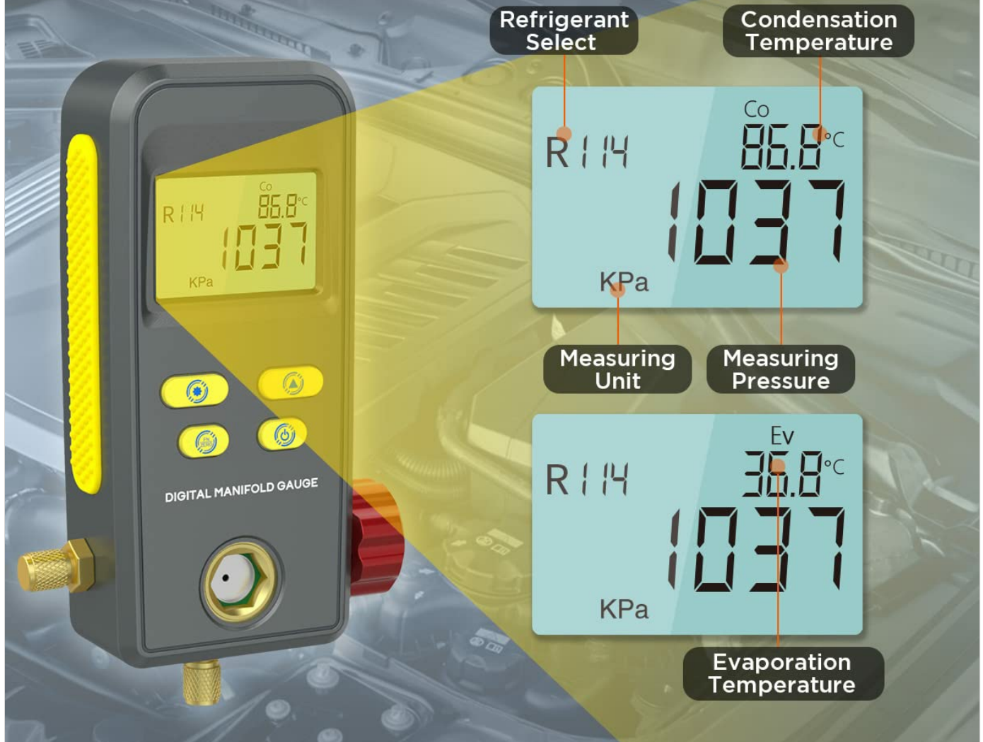
Image: The digital manifold gauge screen showing refrigerant selection (R114), condensation temperature (Co 86.8°C), measured pressure (1037 KPa), and evaporation temperature (Ev 36.8°C) during filling and testing.
