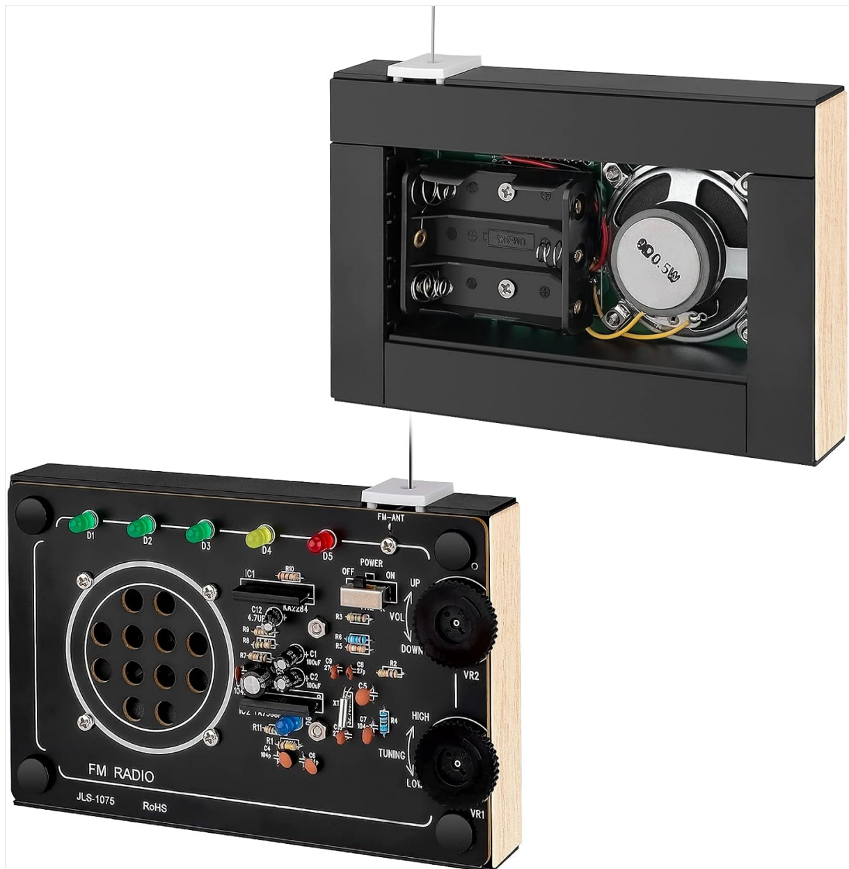
Image: The back of the radio showing the speaker and the battery compartment, indicating how the speaker is mounted.
