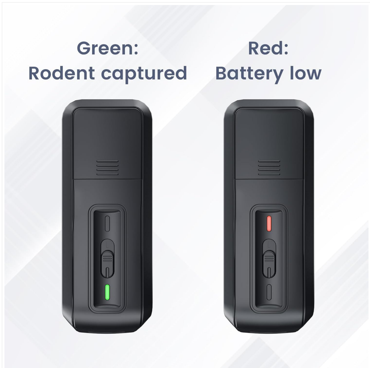
Figure 10: Green light indicates rodent captured, Red light indicates low battery.
