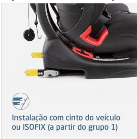
Image: Close-up showing the ISOFIX indicators, which turn green when correctly installed.
