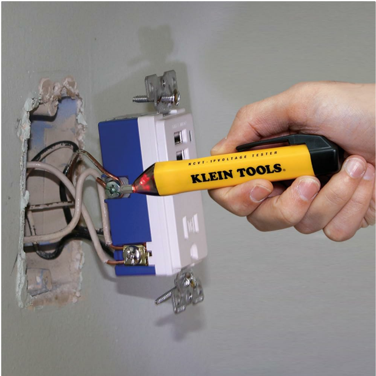
Figure 4: Testing a live outlet. Red LED and audible tone indicate voltage.
