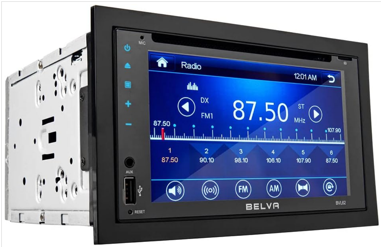
Image 10.1: Radio interface of the BVL62. It shows the current frequency (87.50 MHz), signal strength, and preset buttons for various stations.
