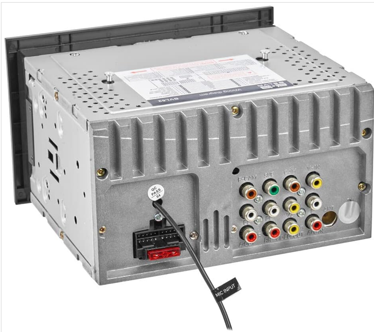
Image 4.2: Rear panel connections of the Belva BVL62. This view shows the main wiring harness connector, RCA outputs for front (FL, FR), rear (RL, RR), and subwoofer (SUB), video inputs (V-IN, CAM), video outputs (V1, V2), and an antenna input.
