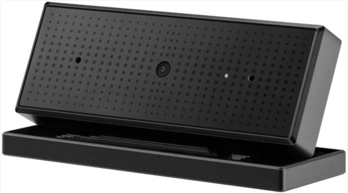
Figure 4.1: Front-top view of the ASUS ROG Eye S, showing the camera lens and the array of AI noise-cancelling microphones.
