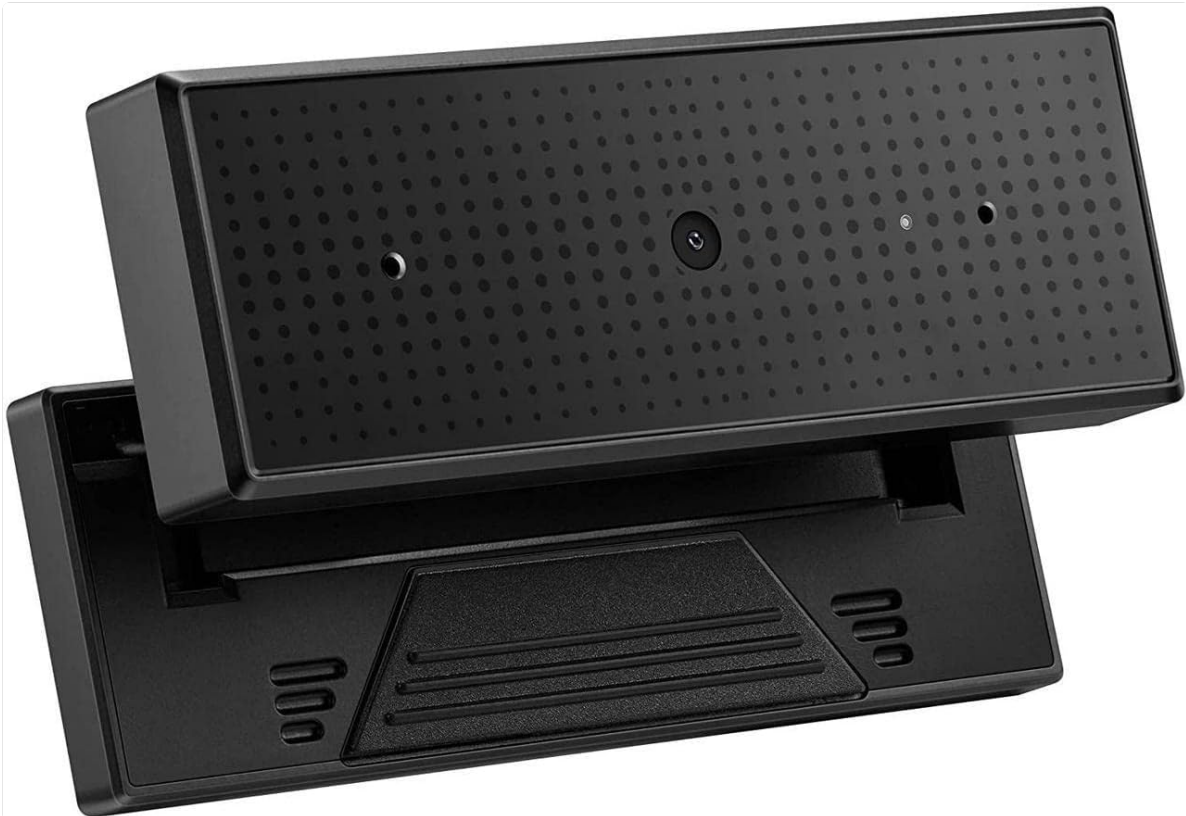
Figure 3.1: The ASUS ROG Eye S webcam in its compact, folded state, ready for placement or transport.
