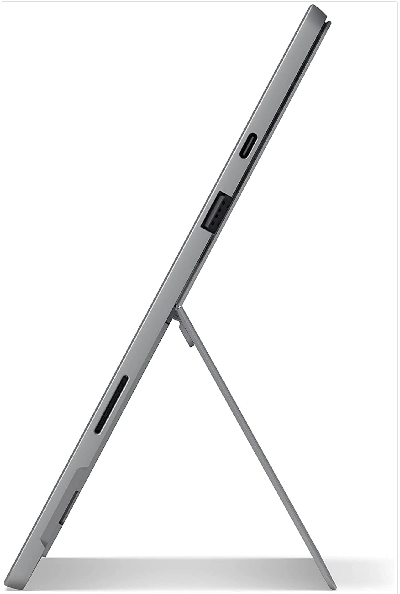
Figure 3: Side view highlighting USB-A, USB-C, and Surface Connect ports.
