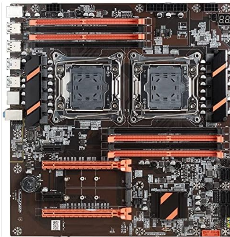
Figure 2.1: Full top-down view of the Atermite X99 Dual CPU Motherboard, showcasing its E-ATX form factor, dual LGA 2011-3 CPU sockets, eight DDR4 DIMM slots, multiple PCIe slots, and various connectors.
