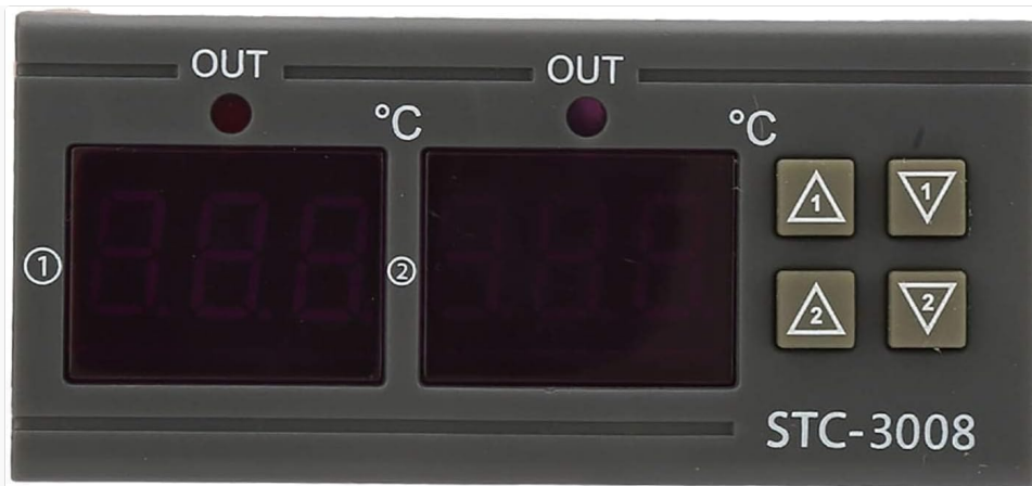
Image 7.1: Front panel of the STC-3008, showing the dual digital displays and control buttons.
