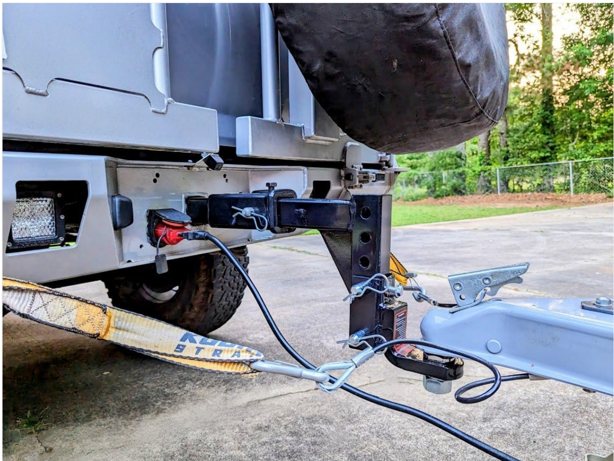
Image 6.1: The TYT Adjustable Trailer Hitch Ball Mount shown with a trailer attached, demonstrating a proper towing setup with safety chains connected.
