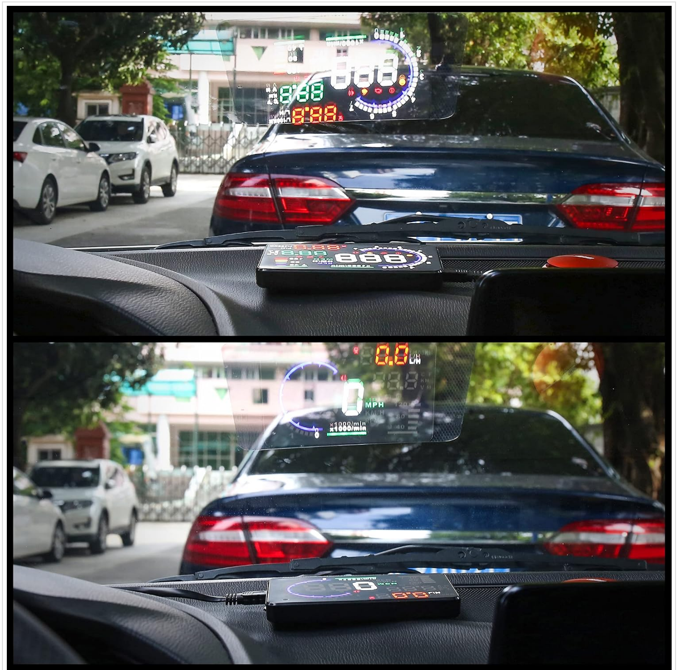
Image 5.1: The HUD unit placed on a car dashboard, showing the projected display on the windshield during daytime and nighttime driving conditions.
